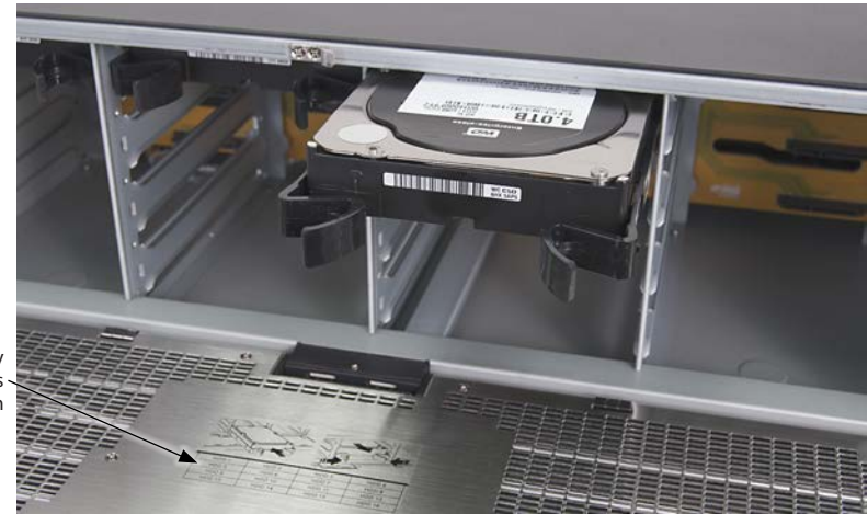
HDD inserted into drive bay
